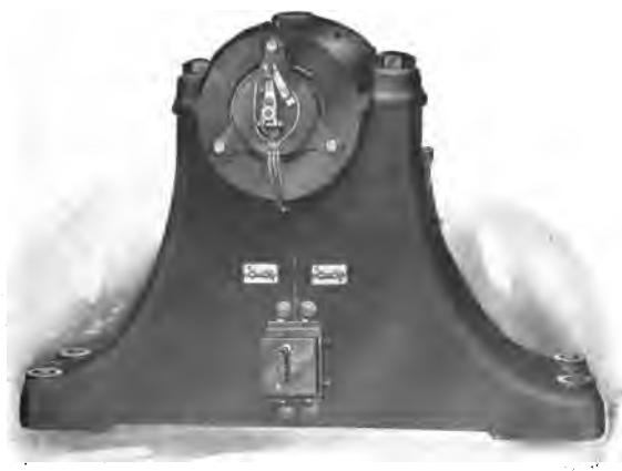
FIG. 341. Electromagnetic end-play device. The General Electric Co.
